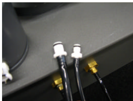
Quick disconnect couplings and o-rings
