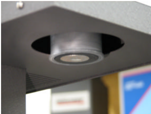
Shroud in Lowest Position
